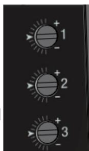
The higher the gain, the more aggressively the helicopter will stop after cyclic movement and the helicopter will feel more stable in the air.
