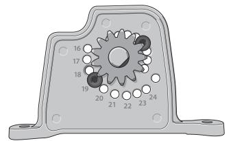
**IMPORTANT:** The included 19T pinion gear is suitable for use with a 6S Li-Po battery.
