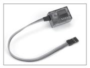
The Flight Log is compatible with the R921X receiver. The Flight Log displays overall RF link performance as well as the individual internal and external receiver link data. Additionally it displays receiver voltage.
