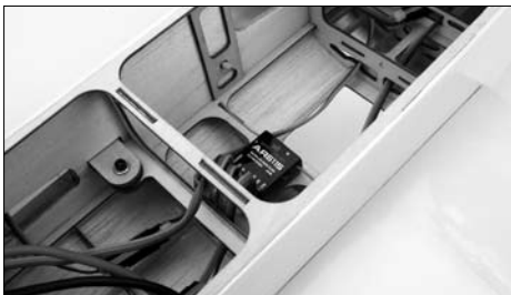
AR6115 installed in airplane
