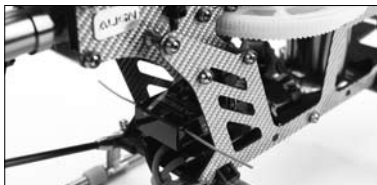
AR6115 installed in Heli
