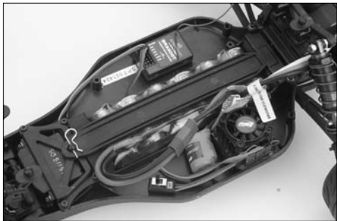
Typical Electric Installation
