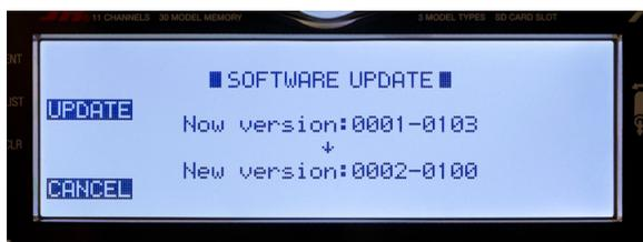
The display will show both your current software version and the new version located on the SD card (for example V0100-0100 to V0002-0100).
