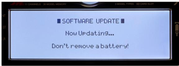
13. The Green LED and screen will remain on during the update. When the first phase of the update is complete (one to two minutes on average), the screen and the LED will turn off.
