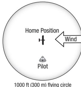
For best performance, compass calibration should be performed before first flight and whenever the aircraft is flown at a new location. Refer to the product manual for complete compass calibration instructions.
