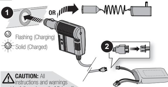
**CAUTION:** All instructions and warnings must be followed exactly. Mishandling of LiPo batteries can result in a fire, personal injury and/or property damage.
