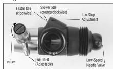
High-Speed Needle: 31/2 turns out (counterclockwise) from closed.
