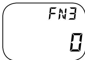
Channel 3 trim adjustment (LN mode only) refer to Channel 3 function, Page 34, for more information
